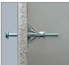
3. Hang the screw head by the special tool (HQ series), then use the tool-gun until the complete opening of the anchor as showed in the picture.
